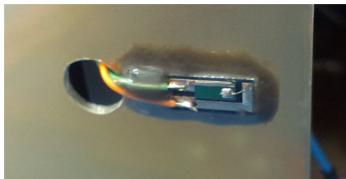
Figure 44: Coarse Sun Sensor Epoxied to Satellite Body
