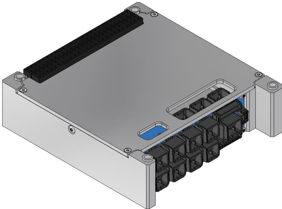
Figure 1: PC104 Variant of CubeADCS
