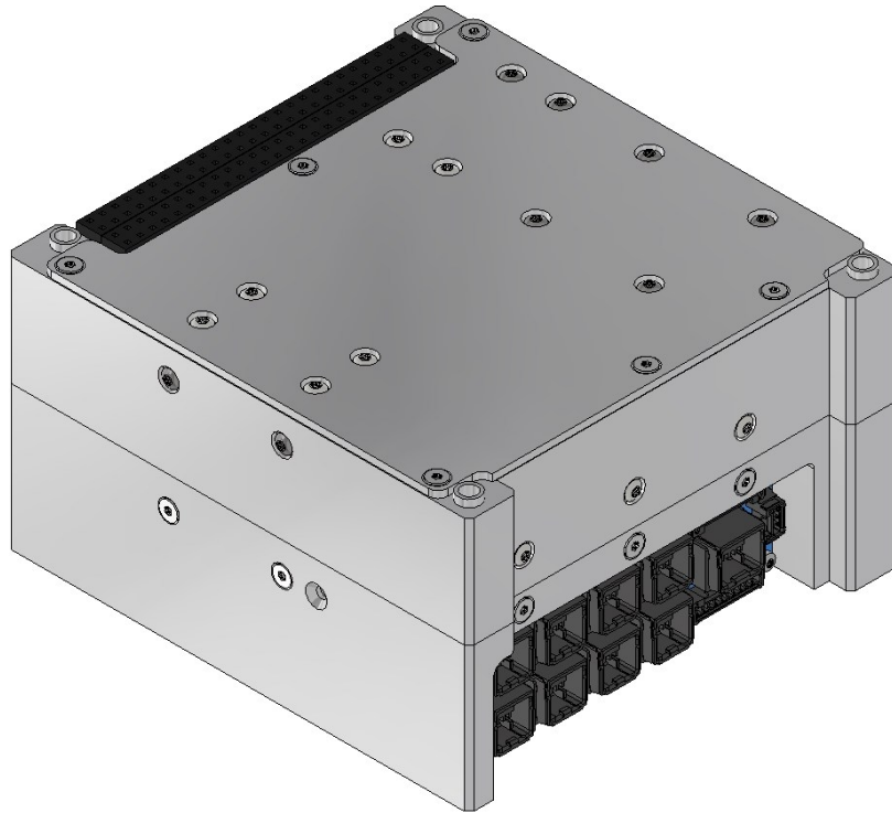
Figure 2: PC104 Variant of CubeADCS for 3U and Smaller Satellites
