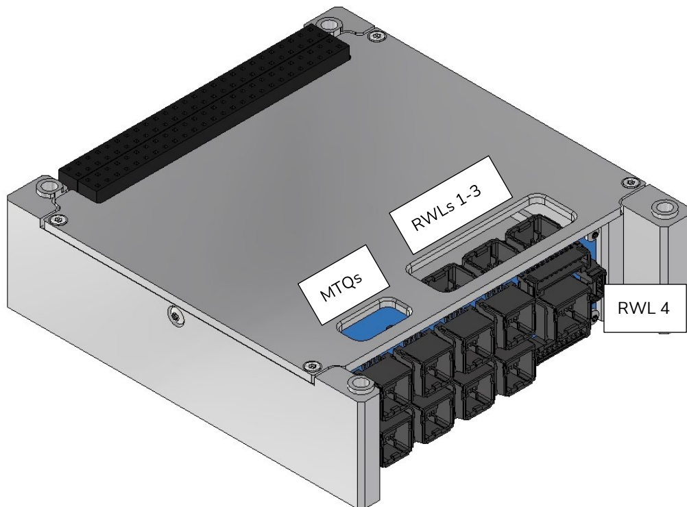
Figure 20: CubeADCS Core (PC104 Variants): CubeConnect Actuator Headers Available to the Outside of Housing
