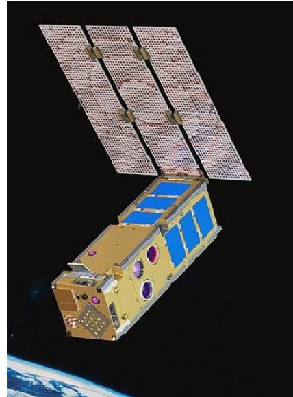
Figure 13: Example of symmetric solar panel layout with small attitude disturbances (left) [image credit EnduroSat] and unsymmetric layout with large attitude disturbances (right) [image credit ESA]
