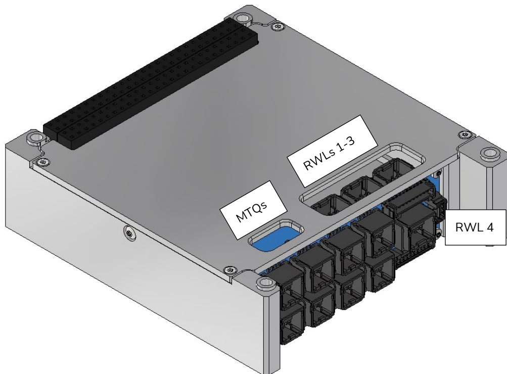
Figure 15: CubeADCS Core (PC104 Variants): CubeConnect Actuator Headers Available to the Outside of Housing
